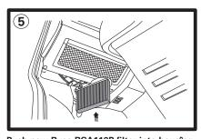
Push new Ryco RCA112P filter into housing.
