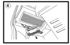
Pull filter cover down and out to remove, pull used filter out from housing.
